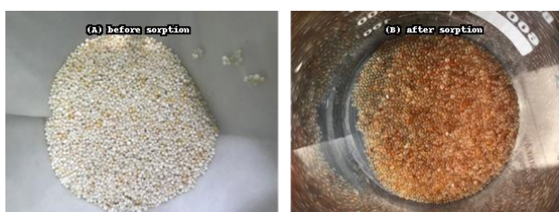
Figure 6 – Visual changes in AMP resin appearance
