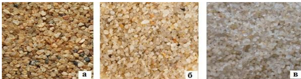
Figure 3 - Photographic images (magnified 100 times) of the initial and beneficiated samples of feldspar-containing quartz sand from the Khiva deposit: a) sample beneficiated by the first method; b) sample beneficiated by the second method; c) sample beneficiated by the third method.
