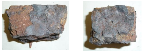
Figure 1.3 – Samples of refractory after operation in the furnace of the cupola
