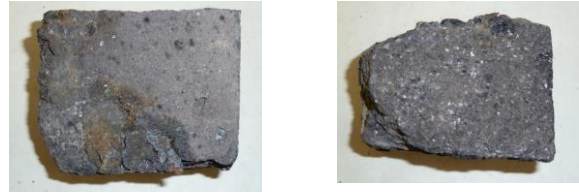
Figure 1.2 – Samples of refractory after operation in the cupola shaft
