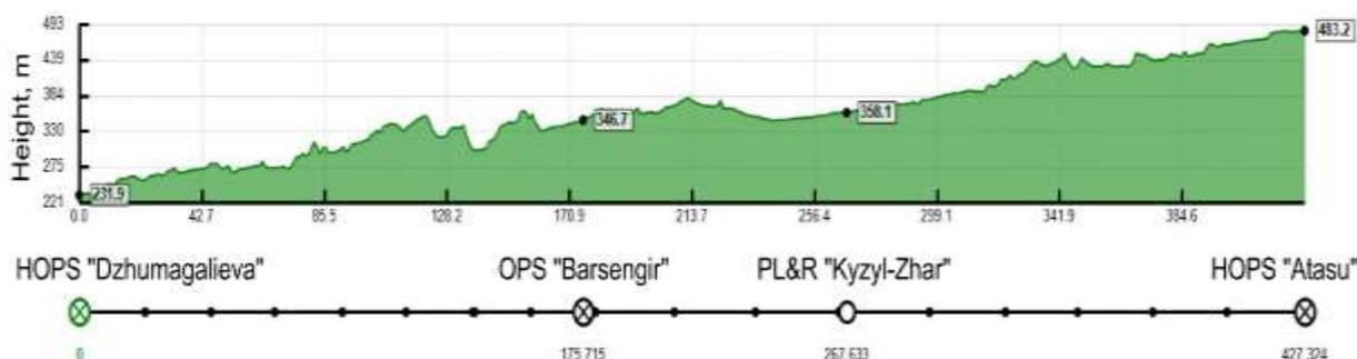
**Figure 3** – Diagram and profile of the Dzhumagaliev – Atasu pipeline section
