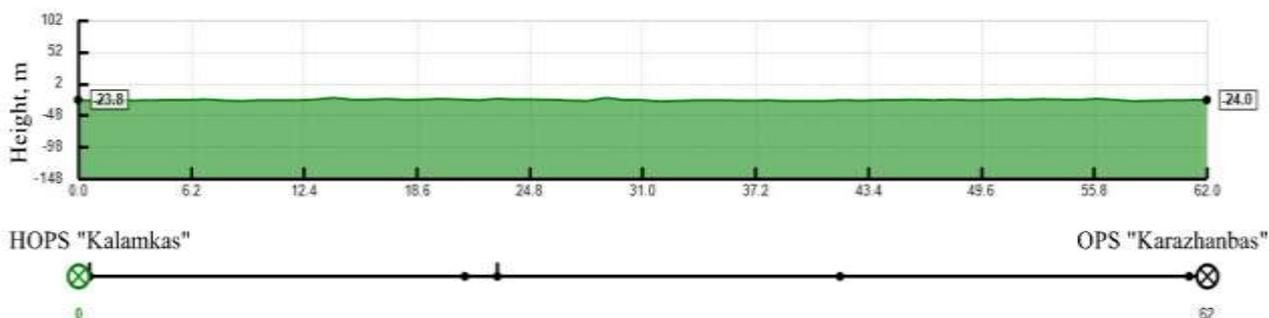
Figure 1 – Diagram and profile of the Kalamkas - Karazhanbas pipeline section
