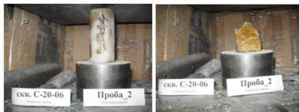
**Figure 1** - Testing of rocks for tensile strength under uniaxial compression on a press
