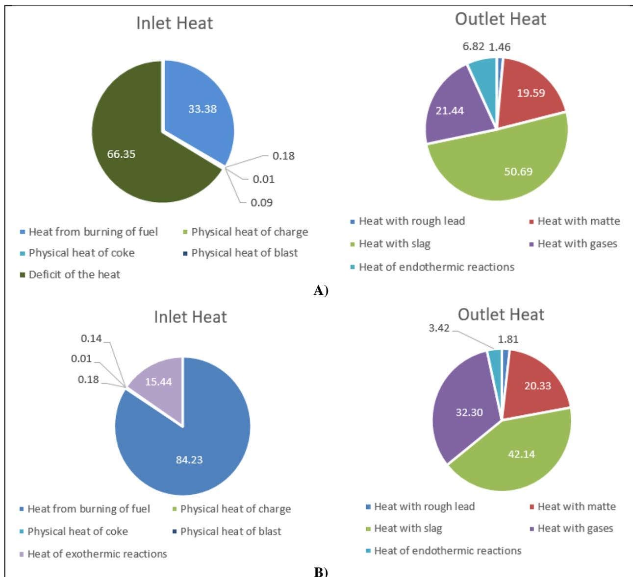
*A) – smelting of charge of existing technology;
