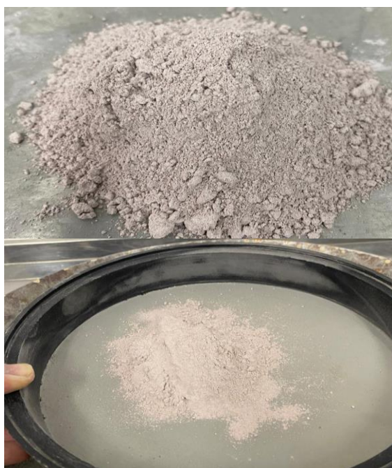
Figure 3 - Determination of grinding fineness of volcanic tuff
