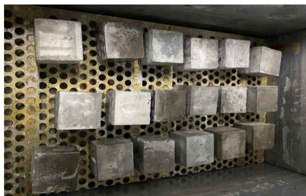
Figure 5 - Concrete samples with CHPP 2 ash as a partial replacement of binder
