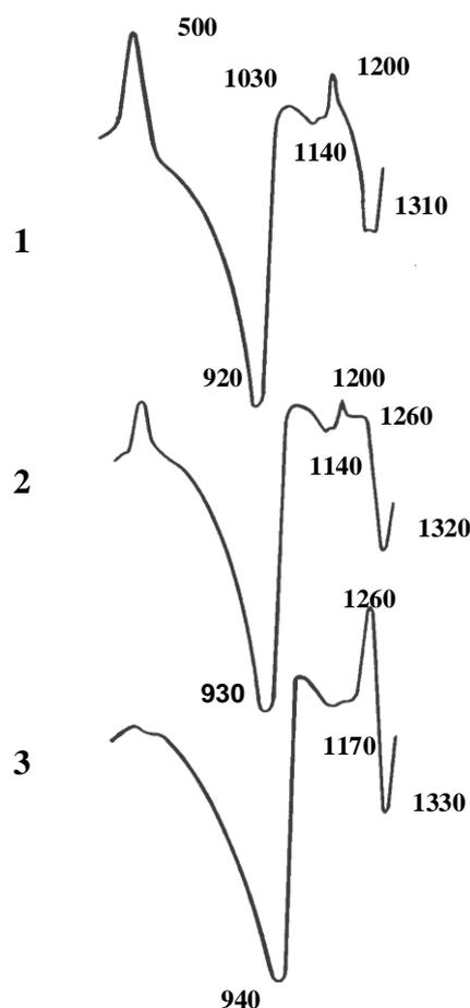
Figure 1 – The DTA curves of raw mixes with various DMS tails content: 1-M type; 2-C type, 3- testing
