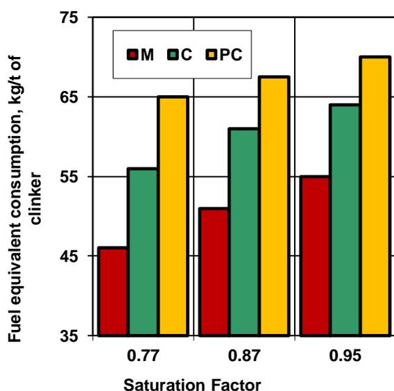
Figure 6 – Specific fuel consumption to the clinker formation for raw mixtures of various content
