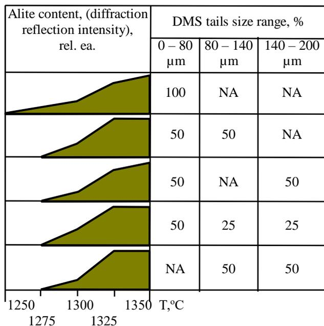
Figure 5 – DMS tails dispersion impact on the clinker phases formation
