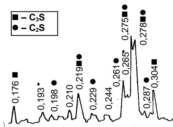
Figure 4 – X-ray pattern of low-basic clinker from the raw mix of M type
