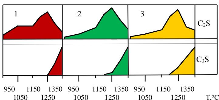
Figure 2 – The clinker phases formation in the raw mixes with various DMS tails content: 1-M type; 2-C type; 3-testing mix
