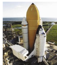
Figure 3 - External fuel tanks and thrust panels of the Space Shuttle tank made of aluminum-lithium alloys 2090 and 2195
