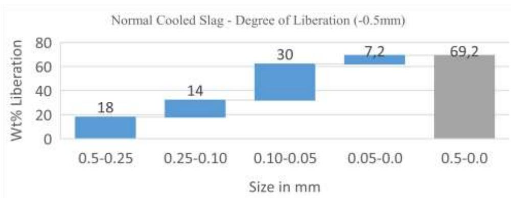
**Figure 13** - Cumulative degree of liberation of normally cooled slag at 0.5mm size
