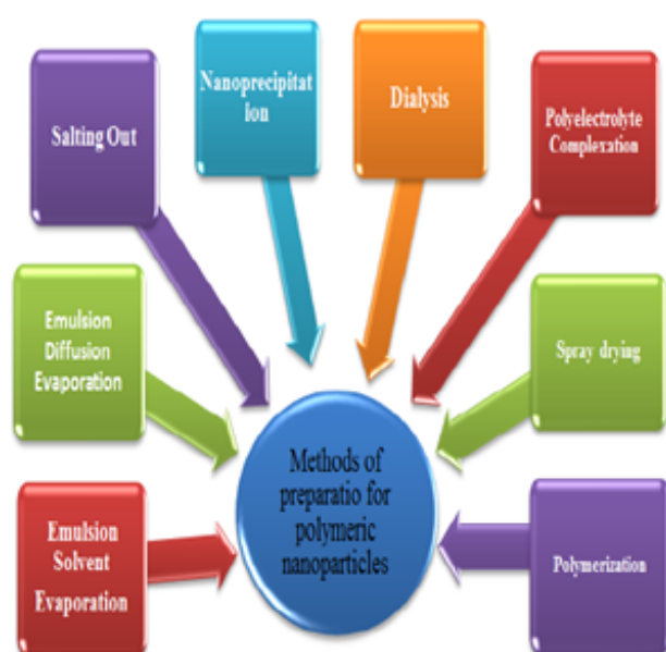
Fig. 15 - Polymeric nanoparticle preparation methods [77]
