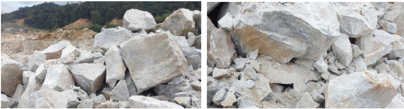
Figure 1 - Results of Limestone Blasting
