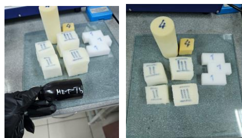
Figure 5 - Polyurethane foam samples and crude oil used.
