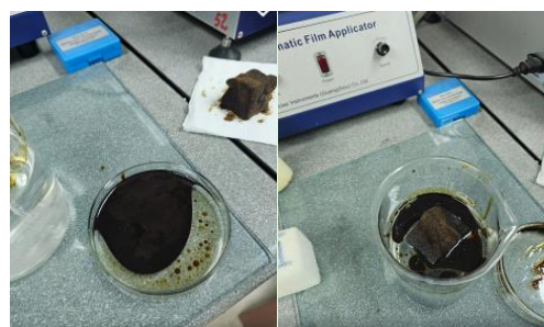
Figure 9 - Oil recovered by mechanical compression.
