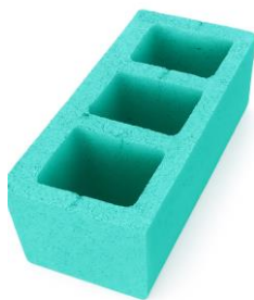
Figure 5 – The building block obtained as a result of extrusion on the installation
