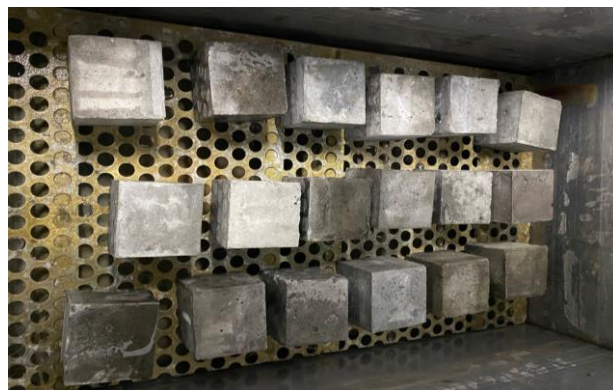
Figure 5 - Concrete samples with CHP 2 ash as a partial replacement of binder
