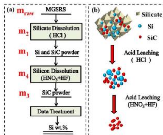
Figure 1 - Schematic diagram of the experiments: a block diagram, b principle scheme [1]
