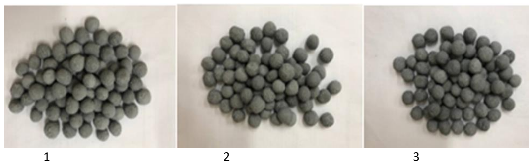
Figure 3 – Ash-slag aggregates with portland cement (sample numbering according to table 2)
