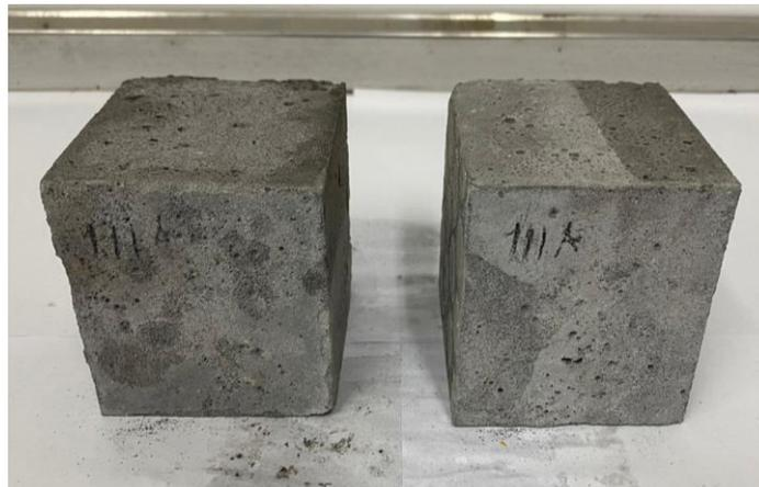
**Figure 5** - Cube samples of ash-concrete without coarse aggregate: composition No 7 with 3% CaCl<sub>2</sub> additive (table 4)
