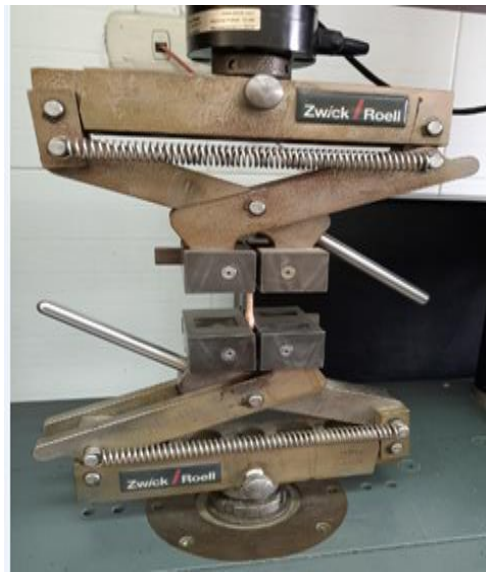
Fig. 12 - 3D printed dog-bone specimens during testing using mechanical testing machine Zwick/ Roell Z010 according to ASTM D638.
