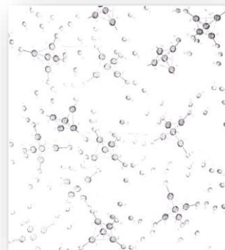
Figure 4 - Scheme of the atomic structure of a eutectic melt of silicon with aluminum (complex eutectic molecules and excess silicon clusters)
