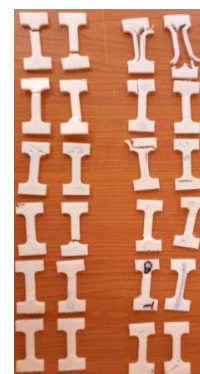
Fig. 13 - The fractured 3D printed dog-bone specimens after testing using mechanical testing machine Zwick/ Roell Z010 according to ASTM D638
