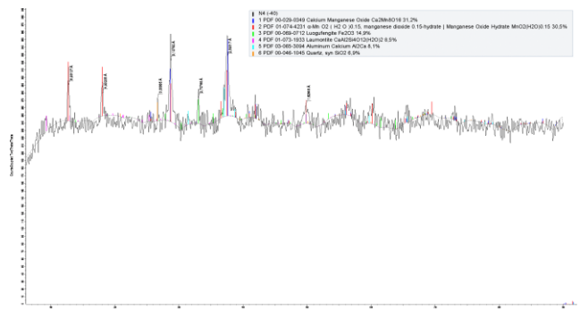
Figure 8 - X-ray diffraction pattern of manganese ores (fraction -40+20 mm)
