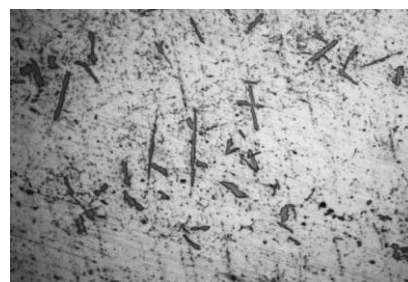
Figure 8 – Microstructures of the Al-Mg-Zr alloys (magnification x200). Series No. 2.
