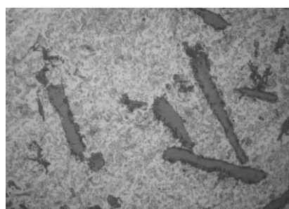
Figure 7 – Microstructures of the Al-Mg-Zr alloys (magnification x200). Series No. 1.
