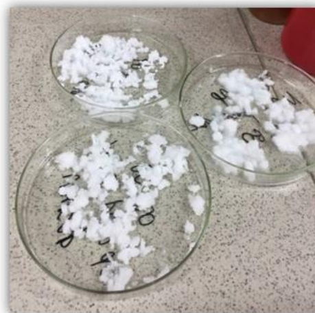
Figure 2 – Synthesized P(mPEG-g-MMA) copolymers
