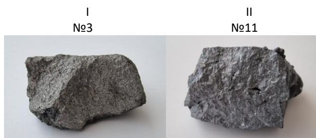
The numbers in the photographs correspond to the melting numbers according to table 3 I- ferrosilicon FS25 (Si=29-32%), II- ferrosilicon FS45 (Si=41.5-43.2%)
