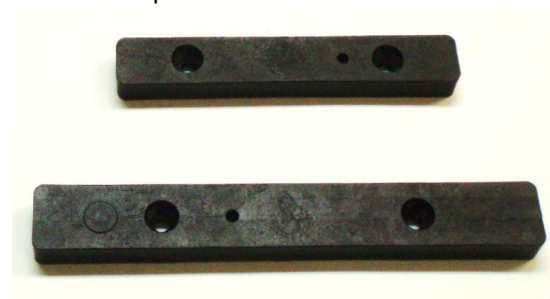
Figure 5 – Guide supports of the MTA-160 crane installation, made of polymer composite
