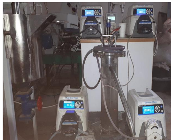
Figure 3 Outotec laboratory thickener 99 mm in diameter
