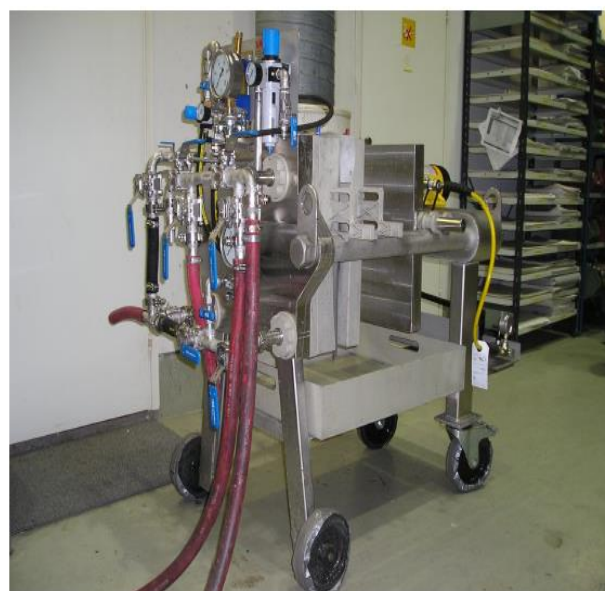
Figure 6 Outotec pilot filter press with 0.27 \text{ m}^2 filtration area.
