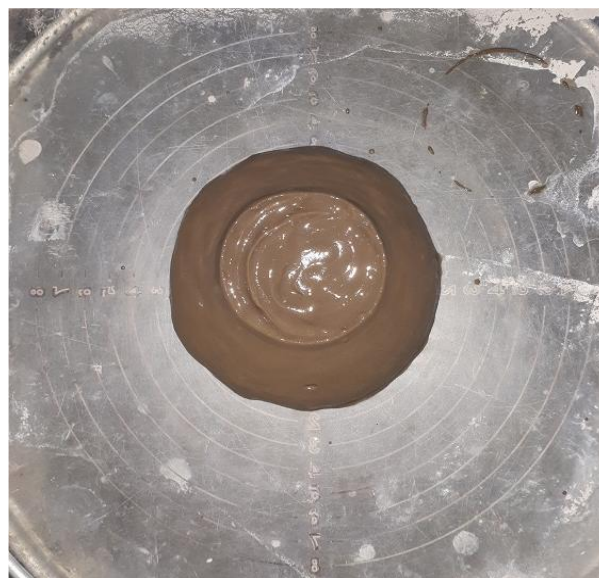
Figure 5 Spreadability of sludge thickened to a 56% density according to the Warman Ring test
