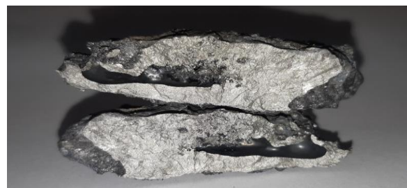
Figure 7 Photograph of a sample of ferroalloy, obtained from the mixture of the first composition
