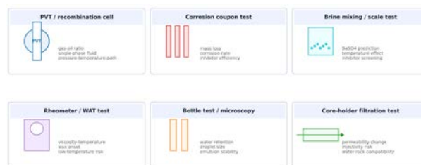
Figure 2 - Laboratory equipment schematic used for integrity-constrained EOR screening
