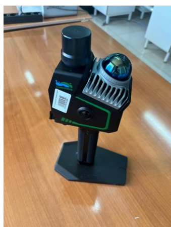
Figure 3 – Handheld LiDAR Greenvalley ARTGEO LIGRIP O2 LITE
