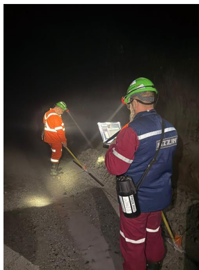
Figure 8 – Process of ground-penetrating radar survey along the floor
