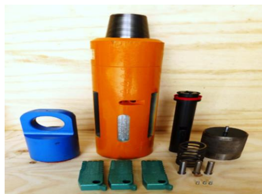
Figure 1 – General view of the U/Reamer MOT 7-1/2 in × 22 in
