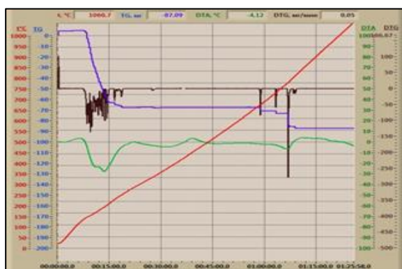
Figure 6 – DTA of the residue obtained during the purification of sodium chloride
