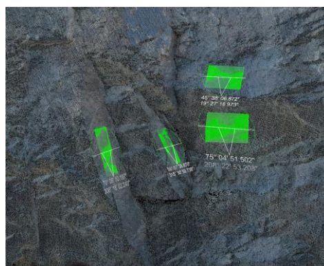
Figure 2 - Measuring process of structural elements geometric parameters
