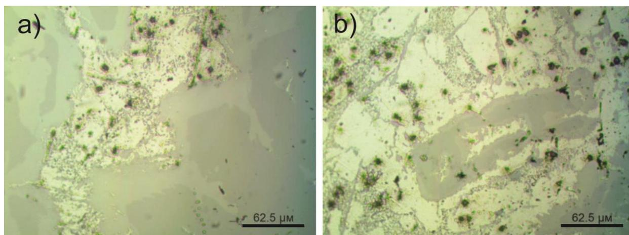
**Figure 2** - Microstructure of AlFeSiMn (a) and AlFeSi (b) alloy, eutectic region
