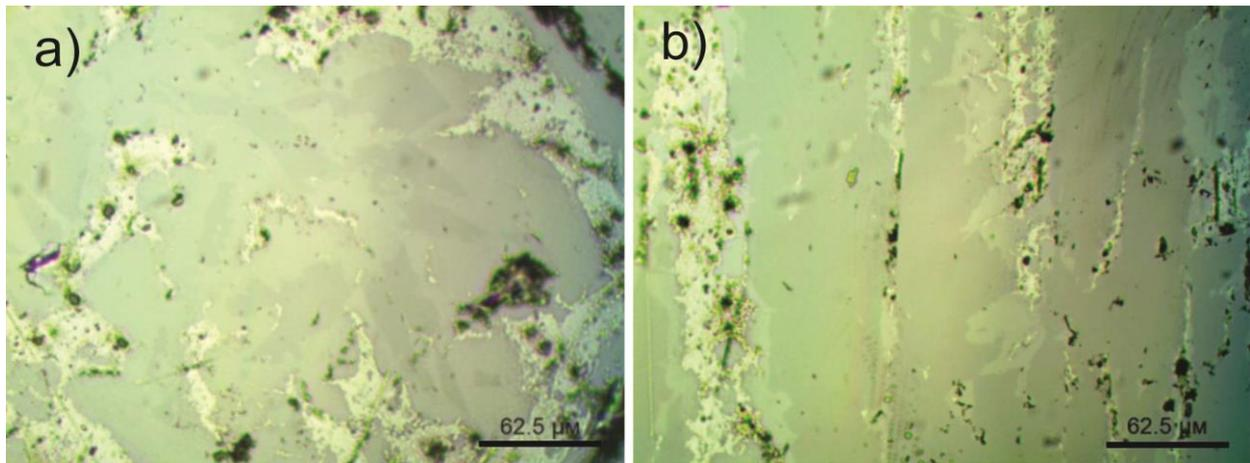
**Figure 1** - Microstructure of AlFeSiMn (a) and AlFeSi (b) alloy, intermetallic region
