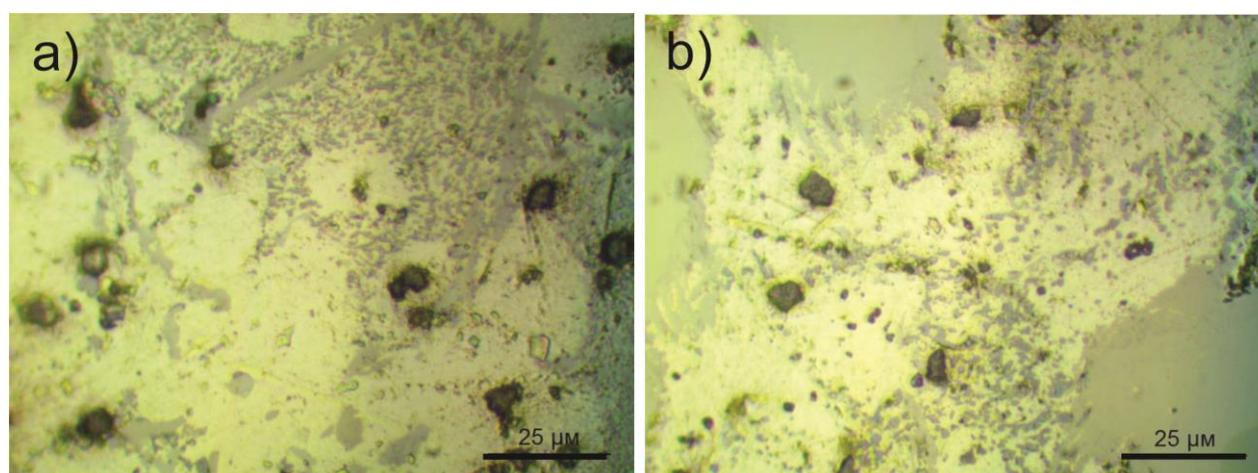
**Figure 3** - Microstructure of AlFeSiMn (a) and AlFeSi (b) alloy, eutectic region (greater magnification)
