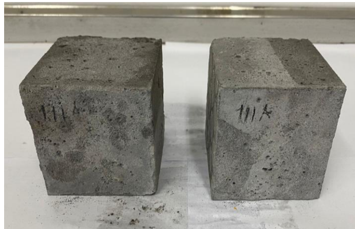
Figure 5 - Cube samples of ash-concrete without coarse aggregate: composition No 7 with 3% CaCl 2 additive (table 4)
