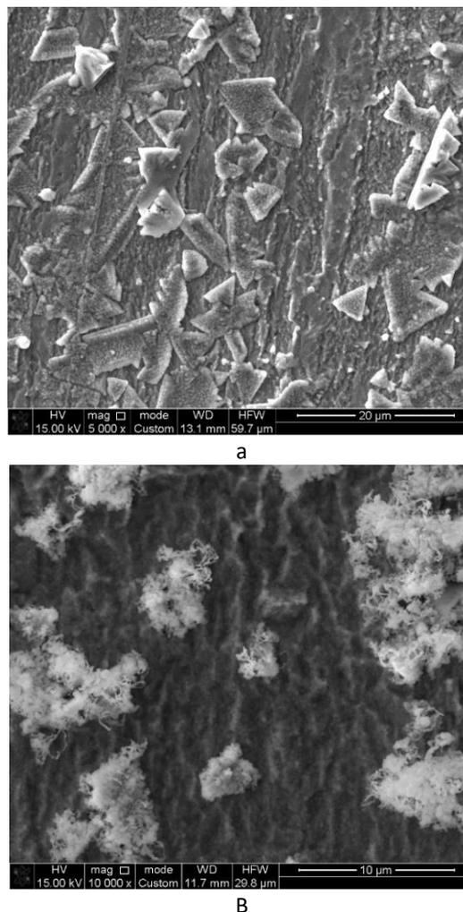
**Fig. 2** - Microphotographs of the surface of a thin silicon film of magnetron sputtering
