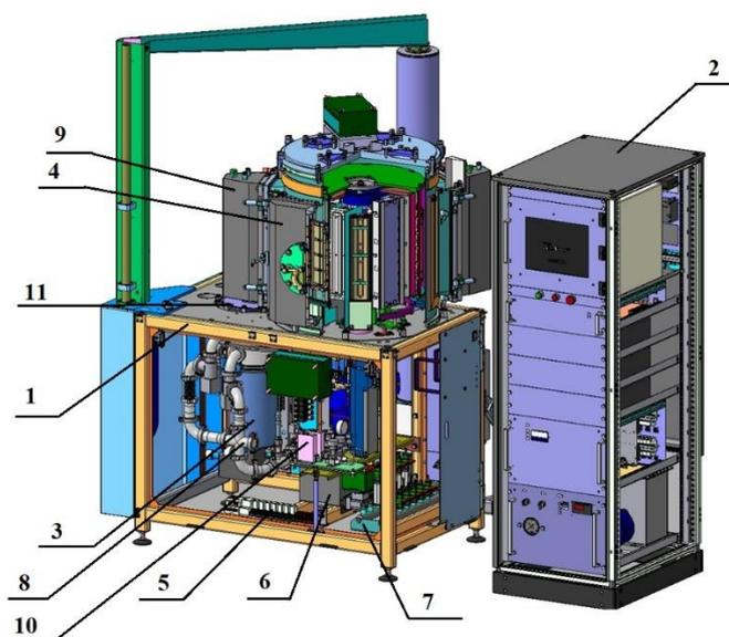
**Fig. 1** - Diagram of the Caroline D12C magnetron sputtering system [6] 1 - technological module, 2 - control cabinet, 3 - fore-vacuum pump, 4 - working chamber, 5 - vacuum system, 6 - pneumatic equipment panel, 7 - water block, 8 - hydraulic equipment block, 9 - lifting and turning mechanism, 10 - gas supply panel, 11 – shutter
