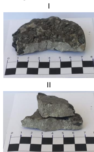
I – 33% of coke, \gamma=20.0\% ; II – 28.5% of coke, \gamma=75\%
