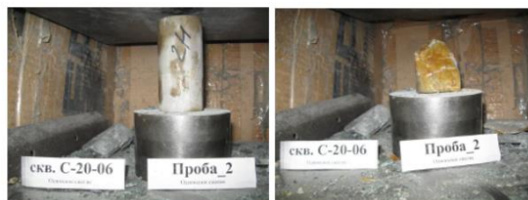
Figure 1 - Testing of rocks for tensile strength under uniaxial compression on a press
