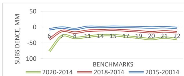
Figure 4 - Plots of benchmark subsidence on the profile line No. 81
