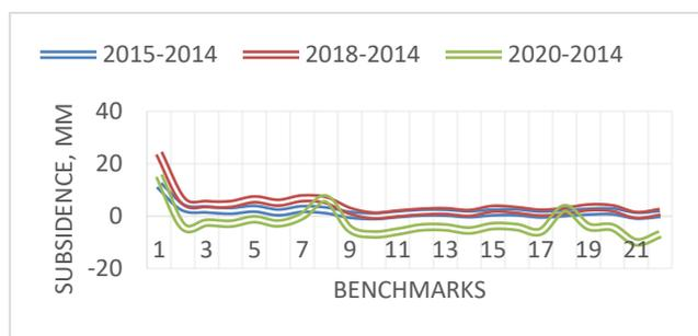
Figure 3 – Plots of benchmark subsidence on profile line No. 80
