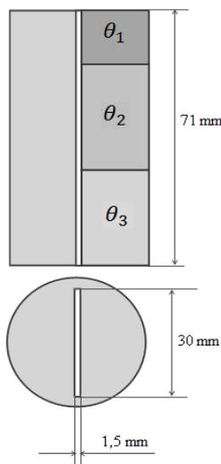
Figure 1 - Diagram of a flat cavity die
