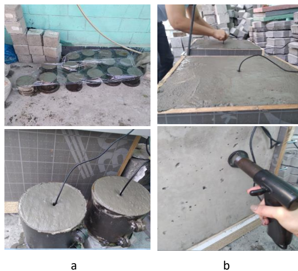
Figure 1 – Experimental studies of specimens: a – SSs, b – LSs
