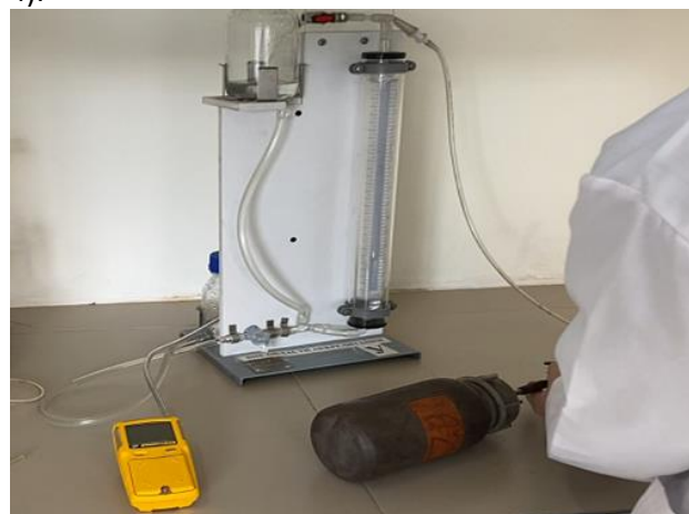
Figure 4. Geokrak desorption unit
