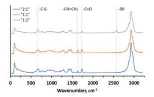
Figure 2 - Raman-spectra of PETriA-EDODET gels with various compositions of the IMM. [PETriA-EDODET] = [2:1], [1:1] and [1:2] mol/mol
