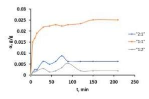
**Figure 4** - Dependence of the swelling rate of PETriA-EDODET gels on IMM composition in distilled water
