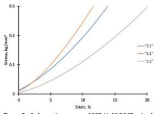
Figure 5 - Deformation curves of PETriA-EDODET gels of various IMM compositions
