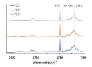
Figure 1 - IR spectra of PETriA-EDODET gels with various compositions of the IMM. [PETriA-EDODET] = [2:1], [1:1] and [1:2] mol/mol
