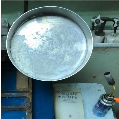
**Figure 6** - Obtaining flake calcium nitrate using a granulator
