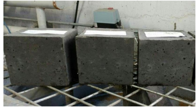
Figure 4 Concrete cube samples
