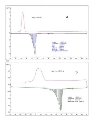
Figure 5 DSC thermograms of mPEG (a) and copolymer P(mPEG-g-VAc) (b)
