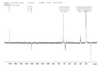
**Figure 4** <sup>13</sup>C NMR spectrum of the obtained copolymer P(mPEG-g-VAc)
