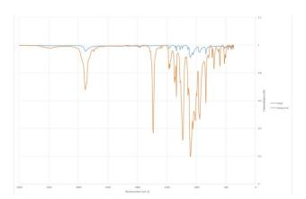
**Figure 2** IR spectra of mPEG and copolymer P(mPEG-g-VAc)
