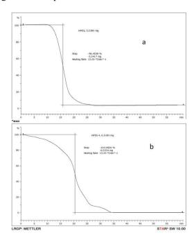
Figure 6 TGA thermograms of mPEG (a) and copolymer P(mPEG-g-VAc) (b)
