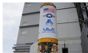
Figure 4 - Centaur upper stage in the Atlas V rocket
