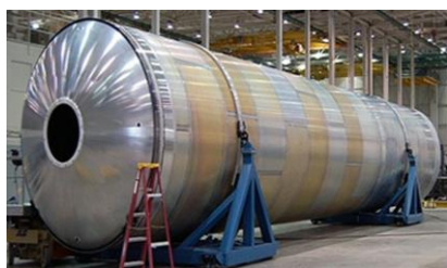
Figure 2 - Falcon 9 fuel tank made of aluminum-lithium alloy 2198
